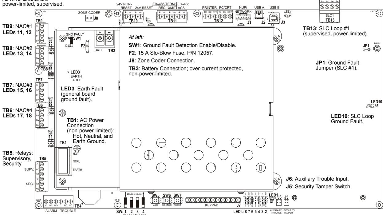
**TB4:** Alarm Relay, Trouble Relay. Output relays; power-limited only if connected to a power-limited source.
