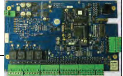
The PRO3000 IP-enabled controller is an advanced access control panel capable of providing solutions for medium to large applications. The PRO3000 provides power and flexibility with its 32-bit CPU architecture, TCP/IP protocol support, flash memory for firmware and large local card holder database.
